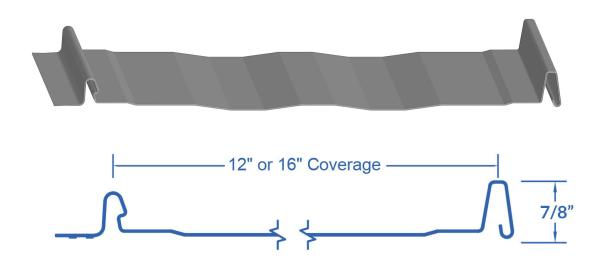
The FormaLoc panel system is a hidden fastener standing seam panel that offers easy installation for roofers and DIY homeowners alike. Available with striations or minor ribs, FormaLoc works well for both roof (26 ga) or side panel applications. With long clean lines, this panel system provides recognized standing seam performance, while remaining an affordable product for a wide array of projects. Forma Loc should always be applied over solid substrate.
